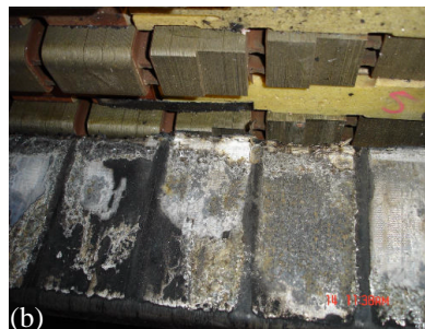
Fig. 5 a. and b. Bars removed from an air-cooled turbine generator suffering from both VS and the loose-coil form of slot discharge.
