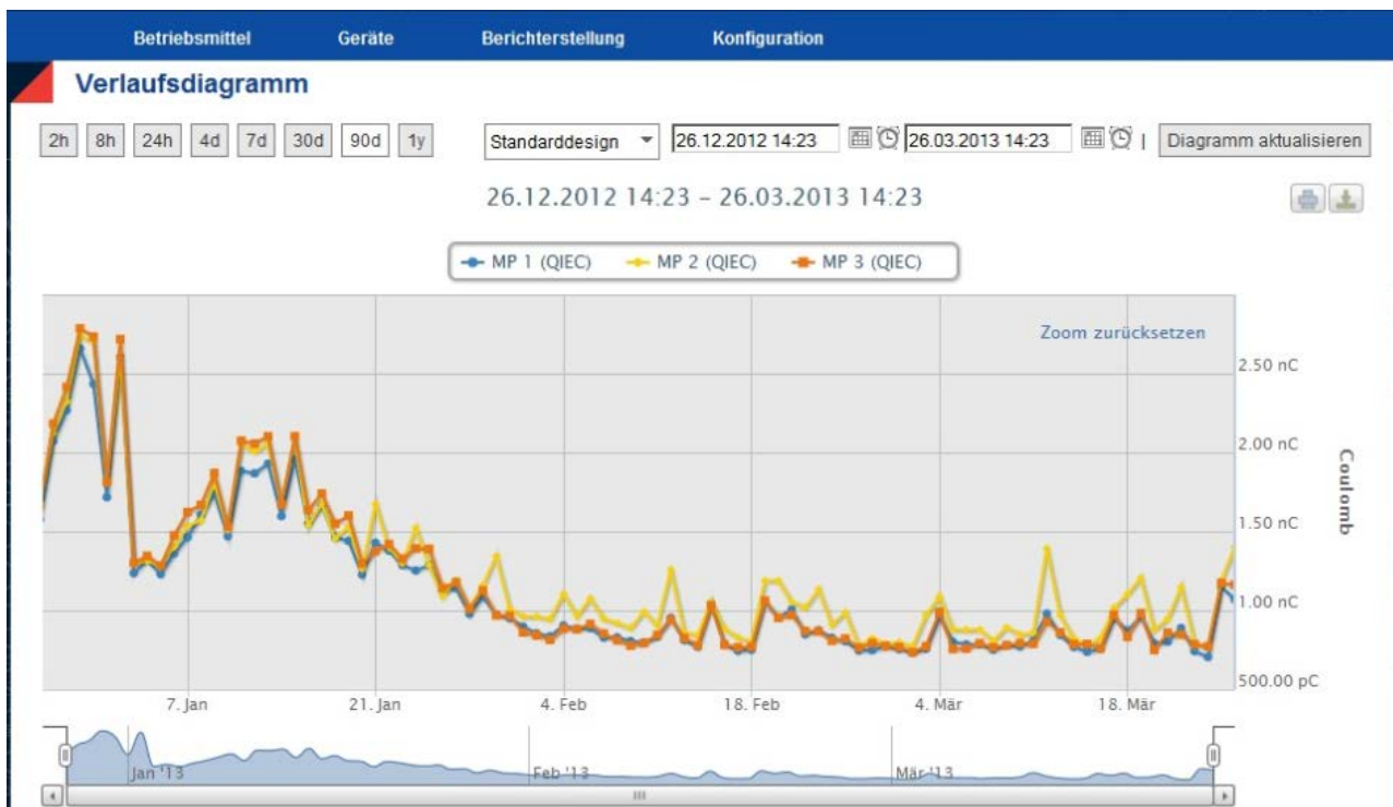
Figure 10 Three phase PD trend diagram
