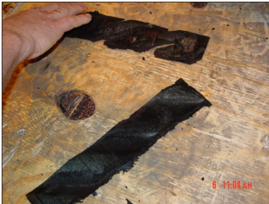
Figure 3-12 Ripple Springs Removed from a Top Bar in the Marshall #3 Unit
