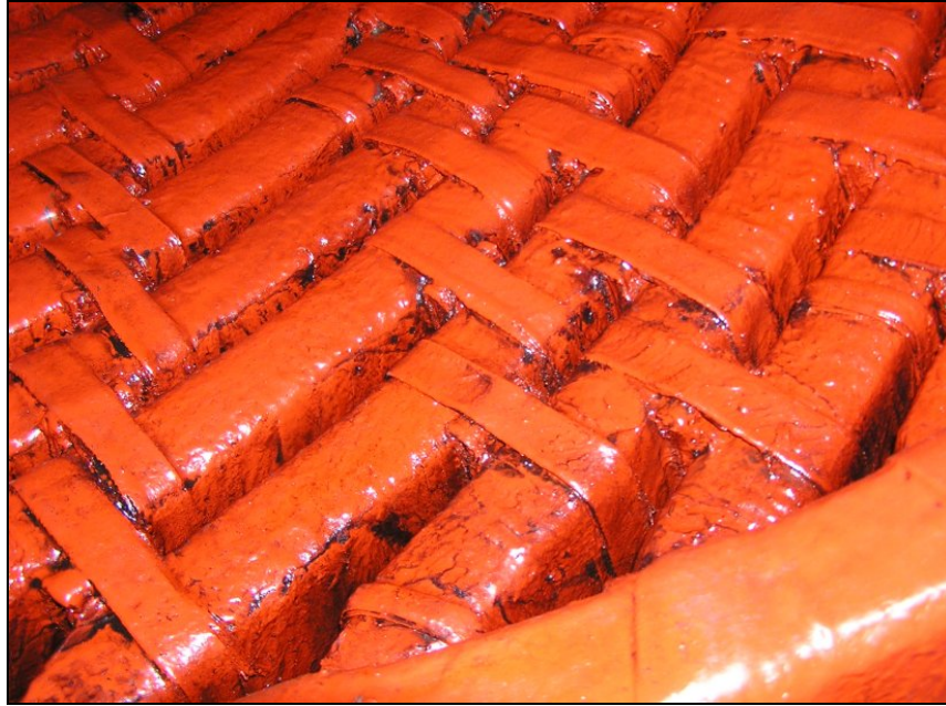
Figure 2-7 Contamination Collecting from Endwinding “Greasing”
