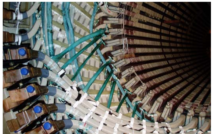
Fig. 4: Top bars mounted over bottom bars.
