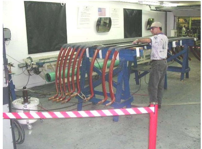
Fig. 9. Testing of stator bars.
