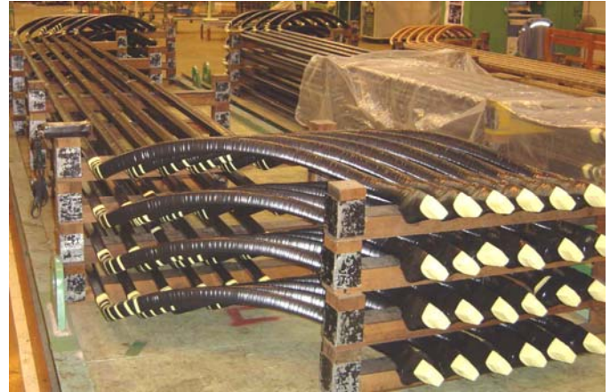
Fig. 2: Both the straight section that fits into the slot in the core iron and the involute that extends beyond the core iron are visible on these coils.
