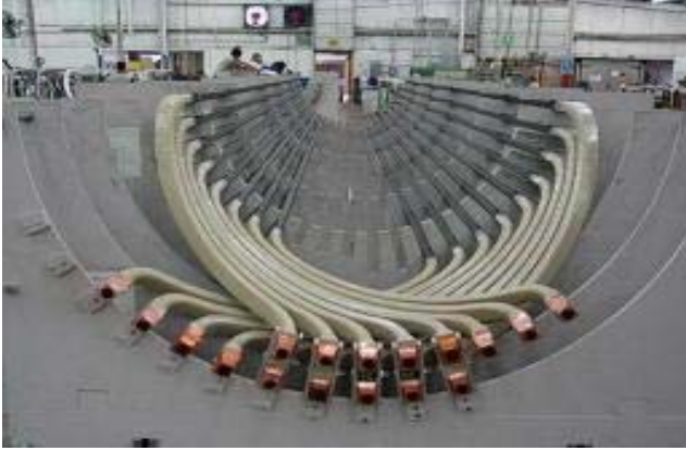
Fig. 7: Mock dummy stator core used to test fit stator bars during manufacturing.
