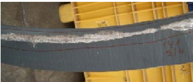
Fig. 8. Spare bars damaged during storage.
