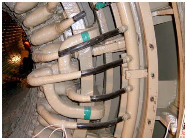
Fig. 5: Water-cooled stator using bar clips.
