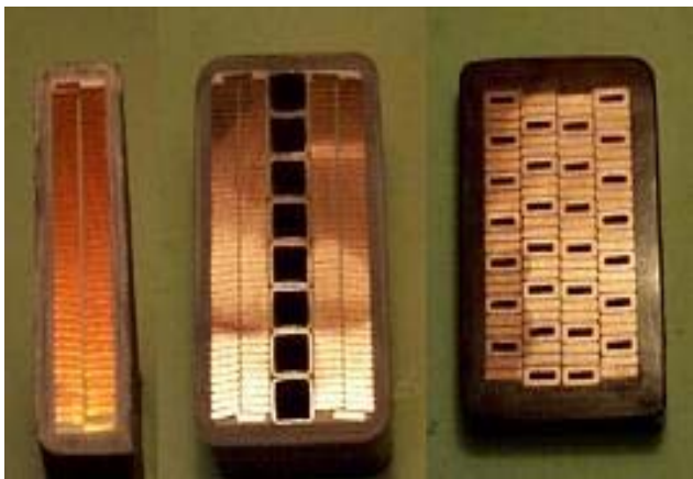
Fig. 1: Typical turbo-generator stator bar cross sections. Left to right: conventional indirect cooled (air or hydrogen), inner hydrogen cooled, and water cooled.
