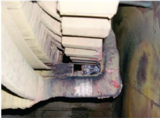
10, 11. Numerous stator-winding failures have occurred in the higher-voltage portions of windings where the ground relay successfully tripped the generator. Repairs to correct the failed phase connection above and the failed series connection at the right were relatively minor
