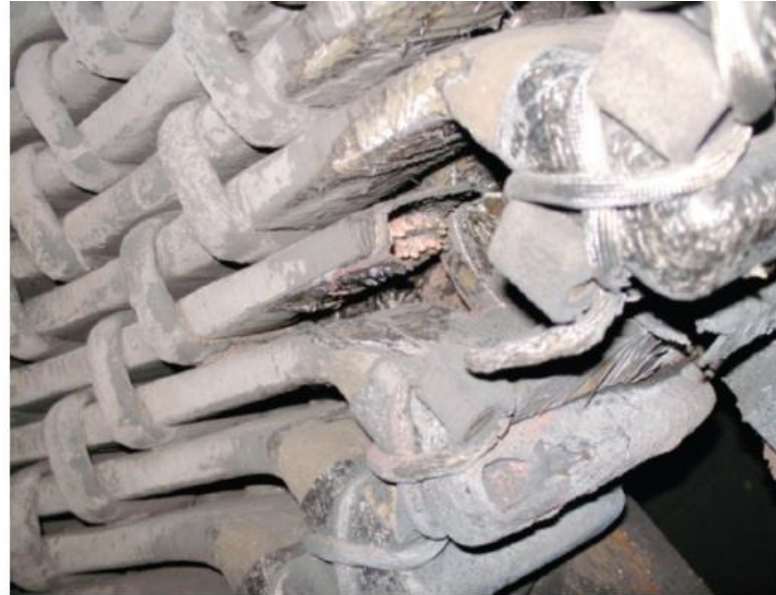
10, 11. Numerous stator-winding failures have occurred in the higher-voltage portions of windings where the ground relay successfully tripped the generator. Repairs to correct the failed phase connection above and the failed series connection at the right were relatively minor
