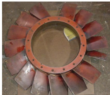
7. Cracking under fatigue. Rotating fans can develop fatigue cracks with enough operational cycles—as this one did. Pieces of blades came loose and caused enough damage to require both stator and rotor rewinds. Courtesy: National Electric Coil
