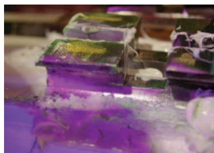
10. Test to prevent cracking. Cracks in a rotor's snap ring groove can be identified by a wet fluorescent magnetic particle test. Courtesy: National Electric Coil
