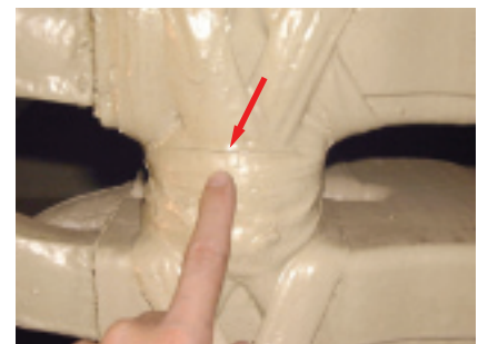
12, 13. Comparing the tiny, but fatal, crack in insulation groundwall at the left with the inconsequential crack from differential expansion at the right illustrates why you want top talent inspecting your generator
