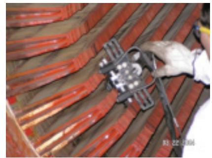
23. EICid search coil and trolley searches for core problems
