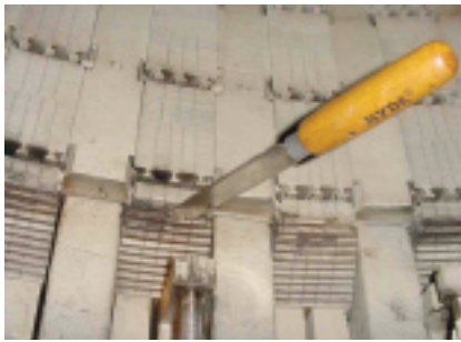
15. Looseness usually occurs at the inside diameter near the ends of the core
