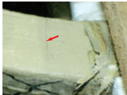
12, 13. Comparing the tiny, but fatal, crack in insulation groundwall at the left with the inconsequential crack from differential expansion at the right illustrates why you want top talent inspecting your generator
