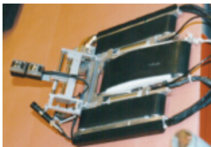
6. Air-gap robot typically carries a camera and wedge-tapper device
