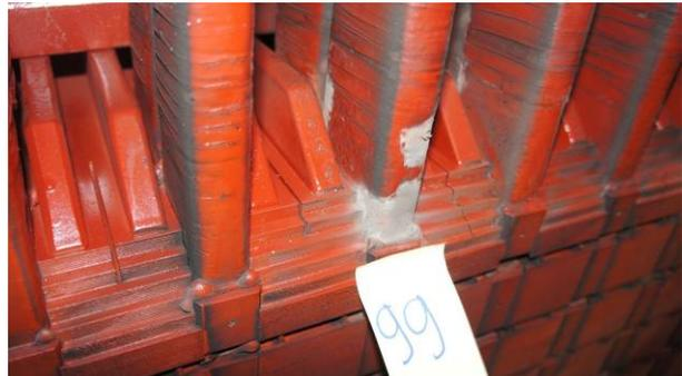
Fig. 33 PD on Cirata Unit 7 slot no.99
