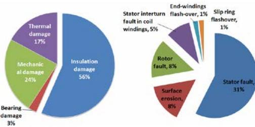
Fig. 2 Occurrence of generator faults [CIGRE 2009 / Survey of Hydro Generator Failures]
