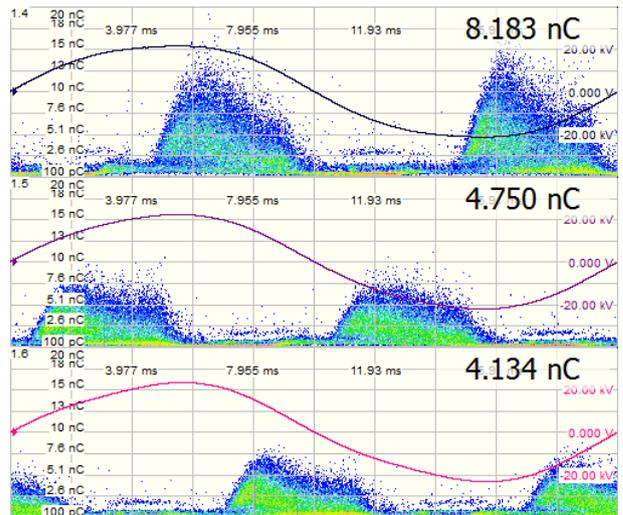
Fig. 20 3-channels PRPD Pattern of cluster 4 (PD between phases)
