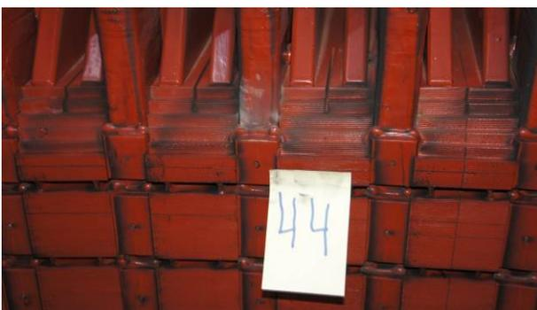
Fig. 31 PD on Cirata Unit 7 slot no.44
