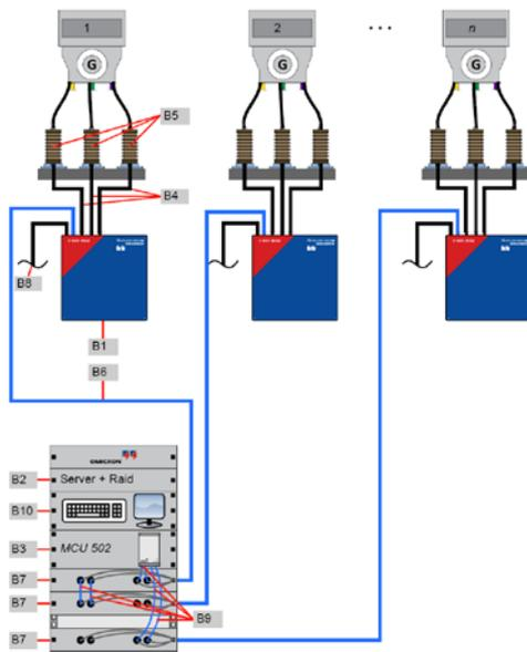
Fig. 3 Continuous (permanent) Monitoring Systems (configuration Principle Example for 3 generator)
