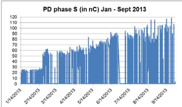
Fig. 6 PD Monitoring data Cirata Unit 7 during 9 months
