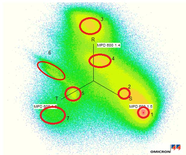
Fig. 10 PD Sources separation using 3PARD
