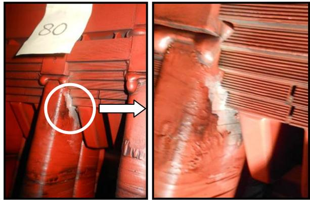
Fig. 32 PD on Cirata Unit 7 slot no.44
