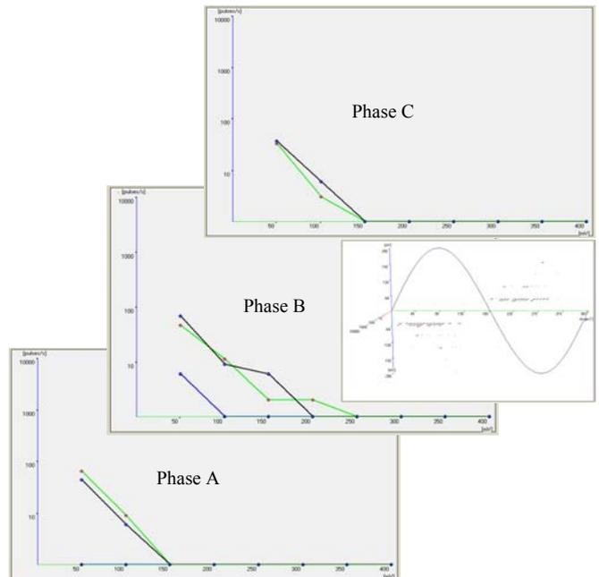
Fig. 5 PD values for 80 vs 500pF couplers at same gain
