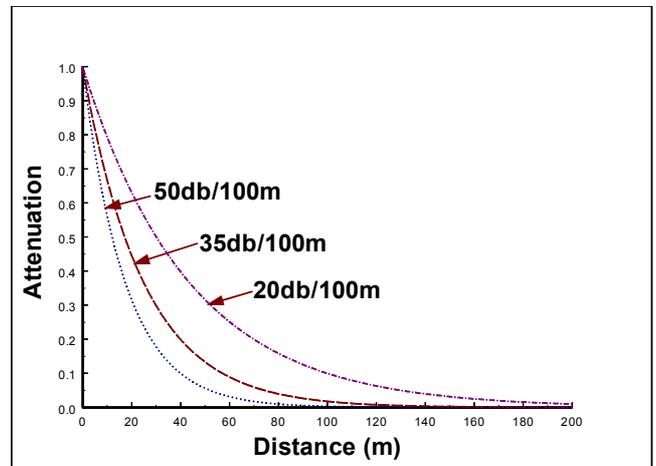
Fig. 2 Attenuation of HF pulses in Power Cable
