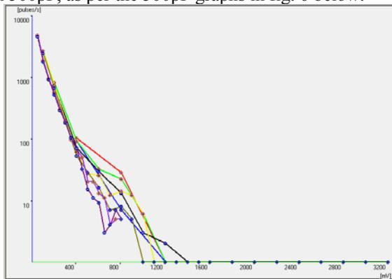
Fig. 6 PD values for 6kV, 500pF, phase B gains 0.25-2.
