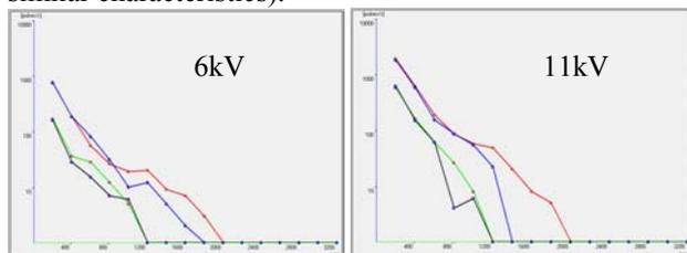
Fig. 7 PD values for 80 and 500pF couplers at 6kV and 11kV.
