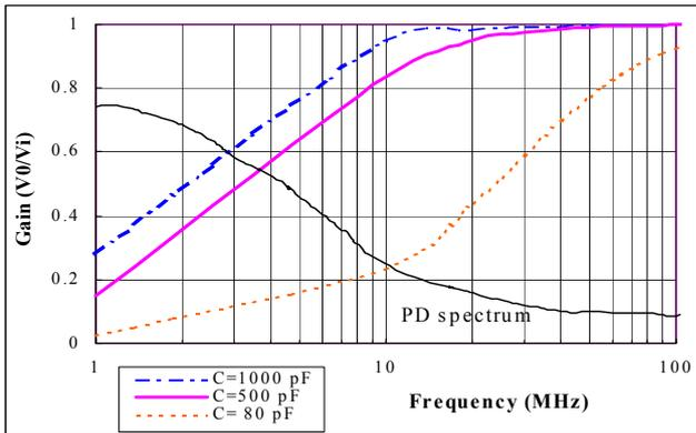
Fig. 3 Frequency characteristics of the detection circuit with various capacitive couplers.
