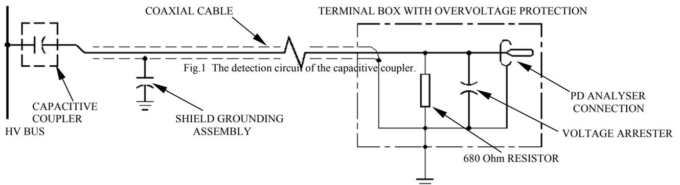
Fig.1 The detection circuit of the capacitive coupler.
