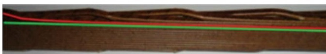
1. Copper strands are Roebel together to form modern mica ground-wall generator bars
