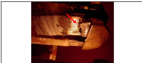
Photo 8. Failure of a parallel one-half bar.
