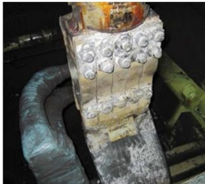
7, 8. Bolted connections improperly made can destructively overheat. Failing flexible lead above connected an HV bushing to isophase bus; HV joint failure at right was caused by loose bolting
