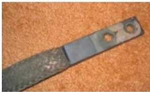
7, 8. Bolted connections improperly made can destructively overheat. Failing flexible lead above connected an HV bushing to isophase bus; HV joint failure at right was caused by loose bolting
