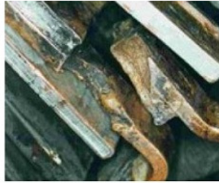
11, 12. Inadequate clearances at phase-to-phase locations difficult to insulate are conducive to failed connections (left). At right is copper burning caused by a non-mica connection insulation failure
