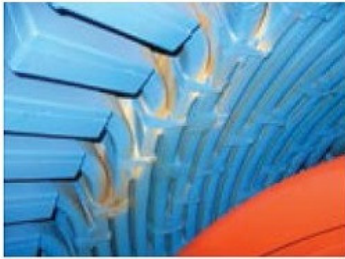
5, 6. Dry ties generally have not performed well in endwinding support systems. At left is dust generated where ties have failed; at right, bare copper is exposed from wear associated with dry ties
