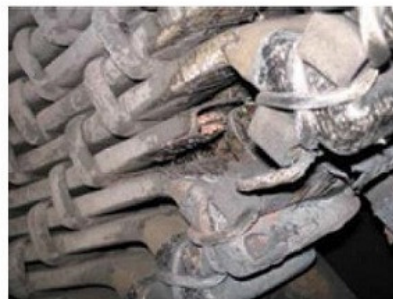
2. Several inches of copper burned away on a stator bar as a result of endwinding resonance
