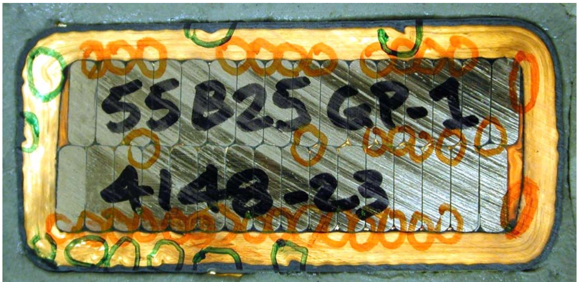
Figure 8 A typical dissection examination of the cross section of a stator bar
