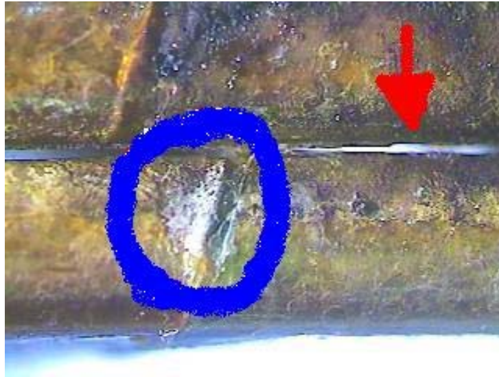
Figure 9 Microscope examination of coil insulation failure
