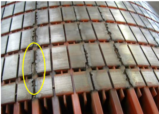
Fig. 13: Damage to an induction motor rotor core due to loose bars in the slot.
