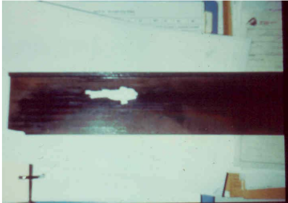
Figure 17: Slot Cell Electrical Failure to Ground
