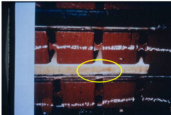
Fig. 4: Destruction of the coil semicon coating in the stator slot due to PD and ozone.
