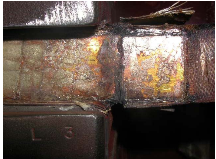
Fig. 12. A close up of the actual turn break in the copper turn.
