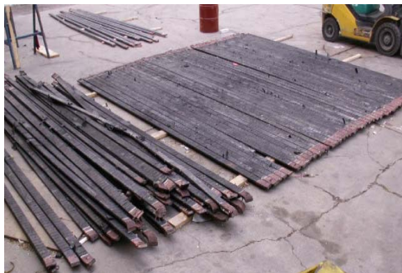
Figure 2. Removed stator bars laid out in sequence for evaluation and inspection.
