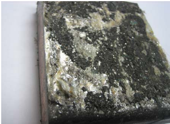
Figure 7. Photo of Stage III Degradation.
