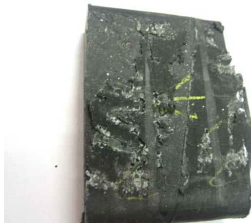
Figure 5. Photo of Stage I Degradation.
