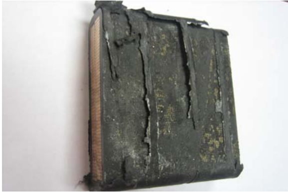
Figure 6. Photo of Stage II Degradation.
