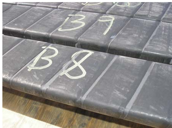
Figure 4. Photo of undamaged bottom bars removed from the original winding.
