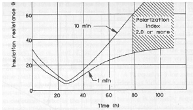
**Figure 6. Dryout Curves for Typical Field Winding**
