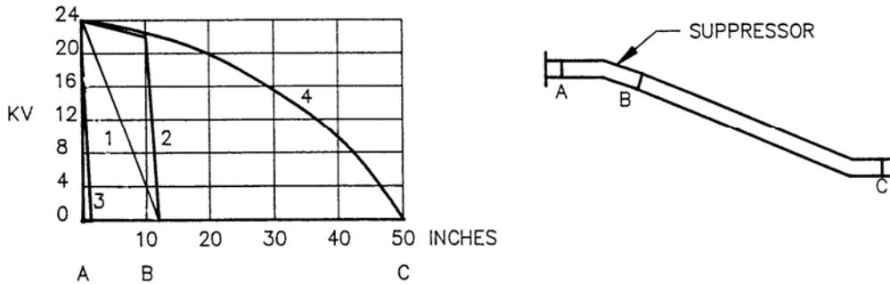
**Figure 2. Approximate Voltage Distribution Across Groundwall Insulation in Stator Bar End Region**
