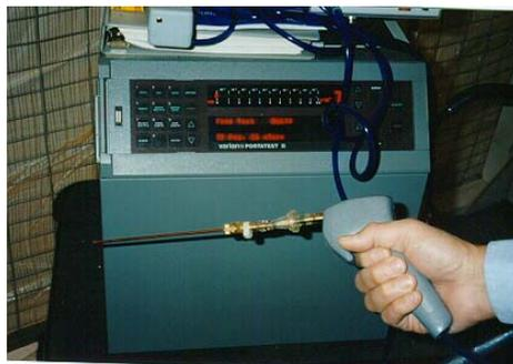
**Figure 28. Gas Test Leak Sniffer and Instrument**
