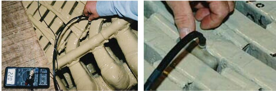
**Figure 34 & Figure 35. Capacitance Testing for Wet Insulation**
