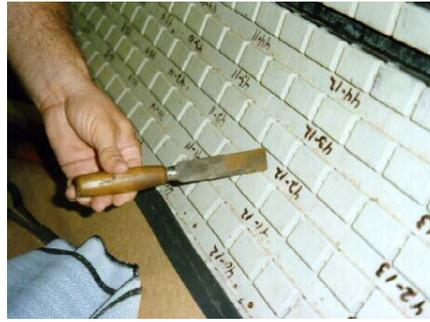
**Figure 24. Knife Test of Core Tightness**
