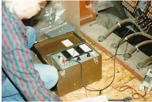
**Figure 21. Instrumentation Measuring RTD Insulation Resistance**
