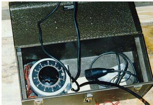
**Figure 15. Power Supply for Measuring Field AC Impedance**
