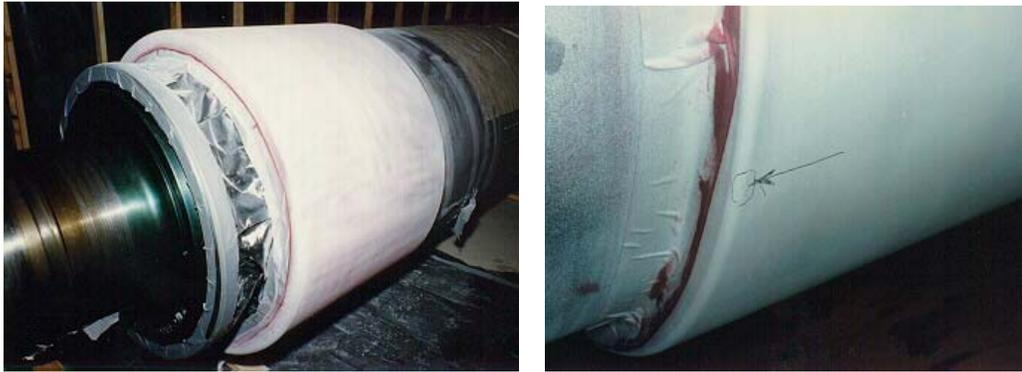
**Figure 13 & Figure 14. NDT Evaluation of Field Retaining Ring**
