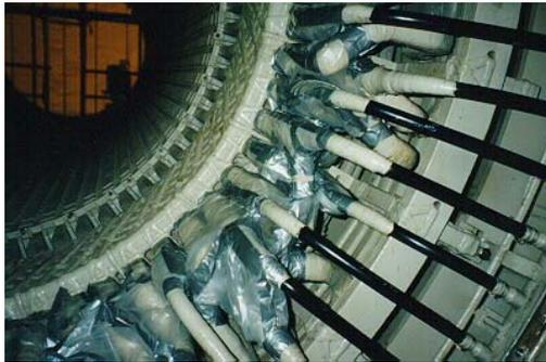
**Figure 33. Bagging of Series Loops for Stator Winding Leak Test**
