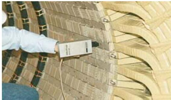
**Figure 12. Hand-held Stator Wedge Mechanical Wedge Tapper**
