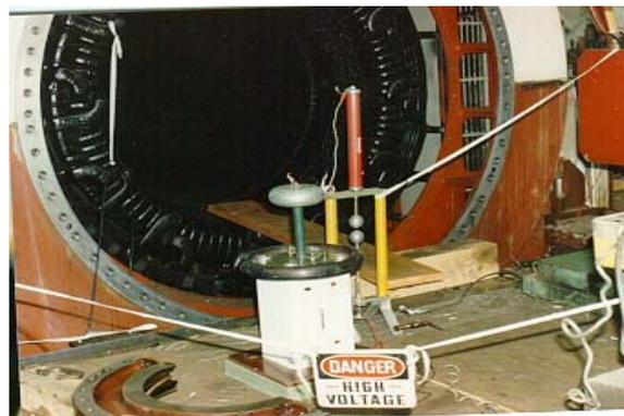
**Figure 8. Inadequate High Potential Test Preparation**
