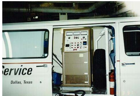
**Figure 4. Van Mounted 0.1Hz High Potential Test Equipment**
