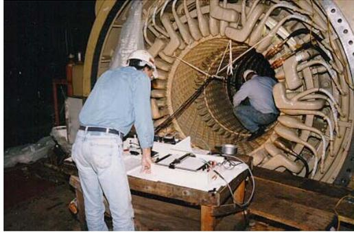
**Figure 22. Low-power Lamination Test Instrumentation and Excitation Coil**
