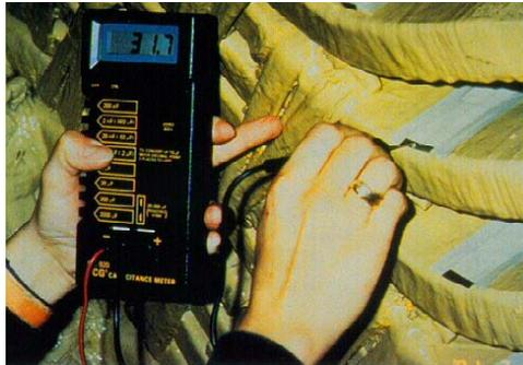
**Figure 29. Bar Insulation Capacitance Testing**
