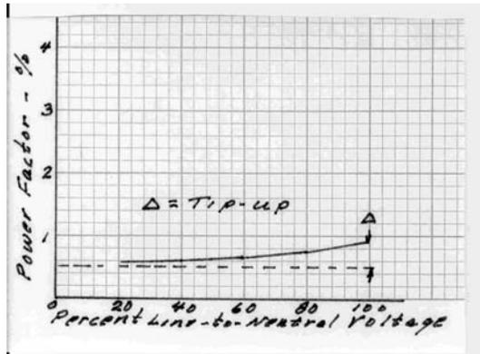
Figure 11. Insulation Power Factor Vs Applied Voltage
