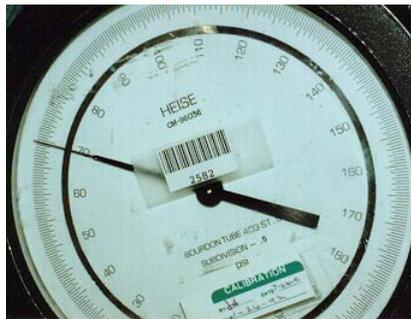
**Figure 27. High Accuracy Pressure Gauge**
