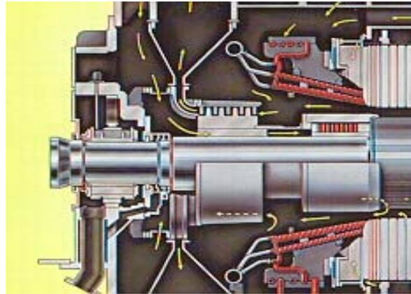
**Figure 23. Flux Shunt Location at End of Core (Westinghouse)**
