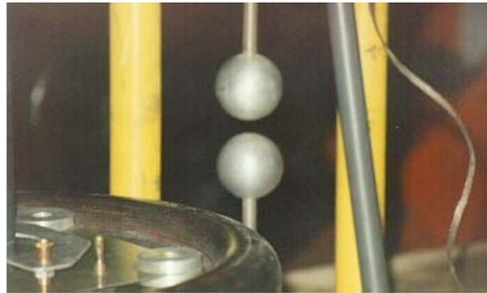
**Figure 7. Sphere Gaps in Use During High potential**
