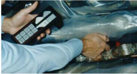
**Figure 32. Checking for Stator Winding Leak using Halogen Gas Detector**
