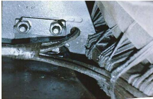
**Figure 9. Stator Winding Support and RTD Cable After Internal Fire Ignited by High Potential Test**
