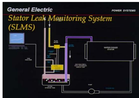
Figure 30. Gas Leak Monitoring Equipment for Stator Windings
