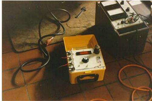
**Figure 20. Digital Low Resistance Ohmmeter (DLRO) on the Left, and Megohmmeter to the Right.**
