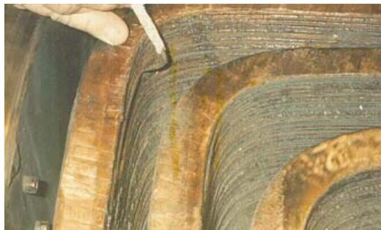
**Figure 18. Field Turn Voltage Drop Test**
