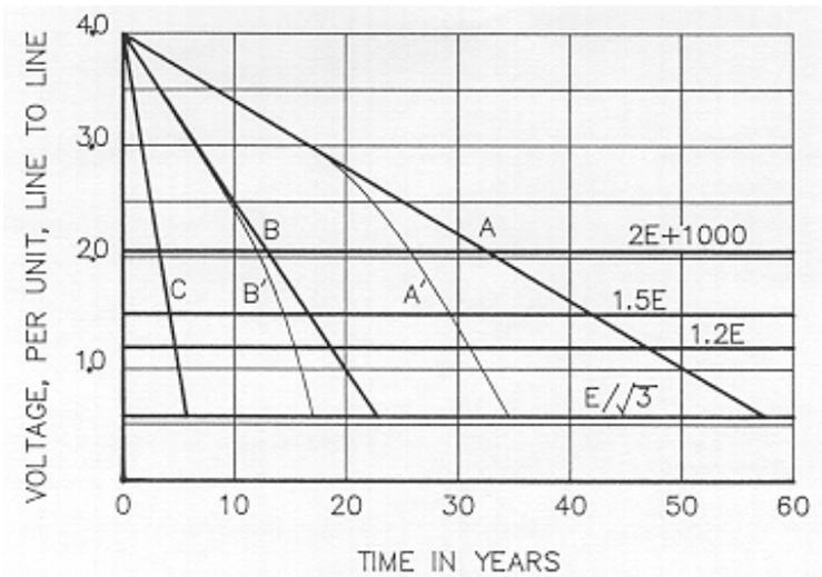
Figure 1. Stator Winding Deterioration Rates
