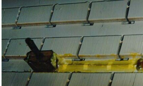
**Figure 19. Assembled Field Turn Short Flux Probe**
